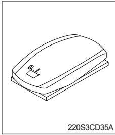
When the switch is pressed ON position, the swing parking brake is locked and swing control is not available by shut off the swing pilot pressure to the swing spool.
